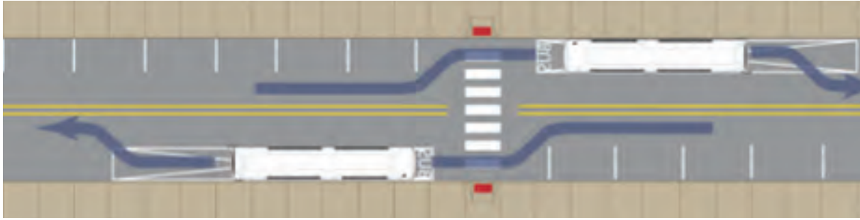
Figure 37a Placement of pedestrian crossing behind bus stops (Southeastern Pennsylvania Transport Authority 2012)
