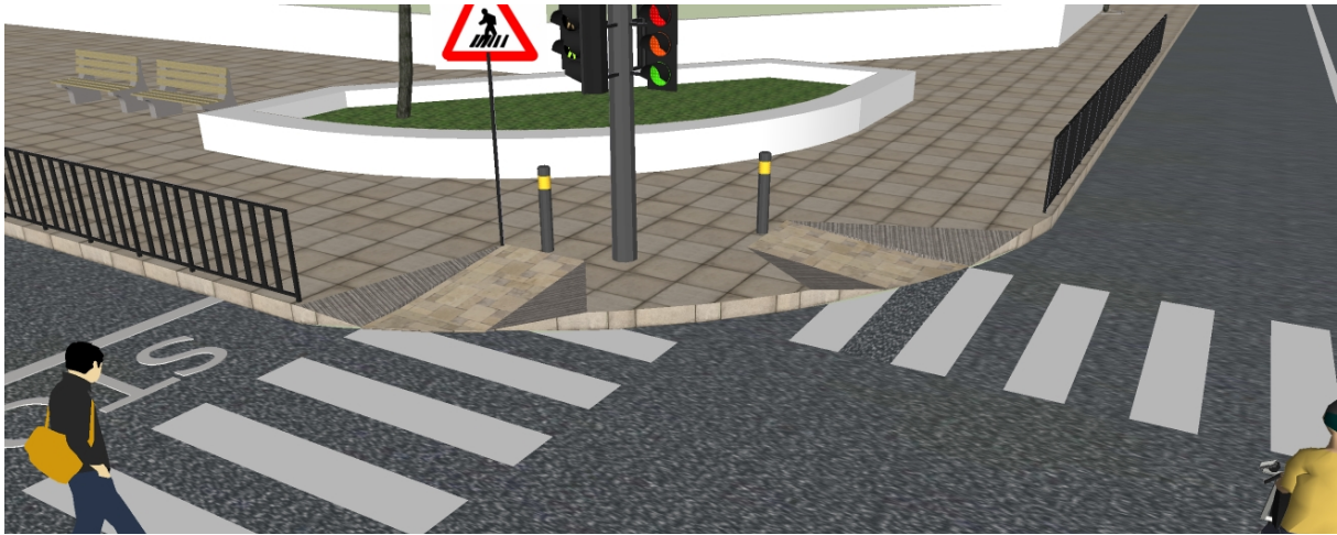
Figure 40 A tighter kerb radius at the intersection can reduce over-speeding (EMBARQ India 2014)
