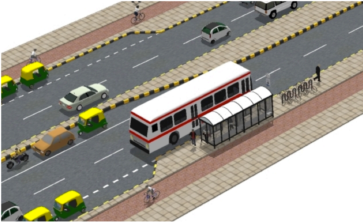
Figure 41 Extension of the kerb at the bus stop can make it easier for the bus to pull up closer to the stop (EMBARQ India 2014)
