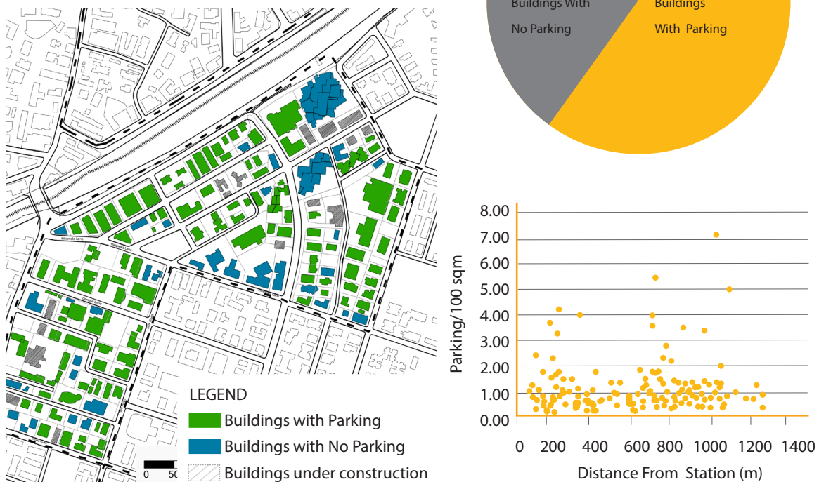
Figure 31: Map (left) and graph (right) showing parking supply, and (bottom right) graph showing parking supply by distance from transit in Block 2; Source: EMBARQ India
