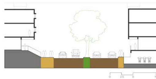
Fig33: Double road and CMH Road : Existing Section
